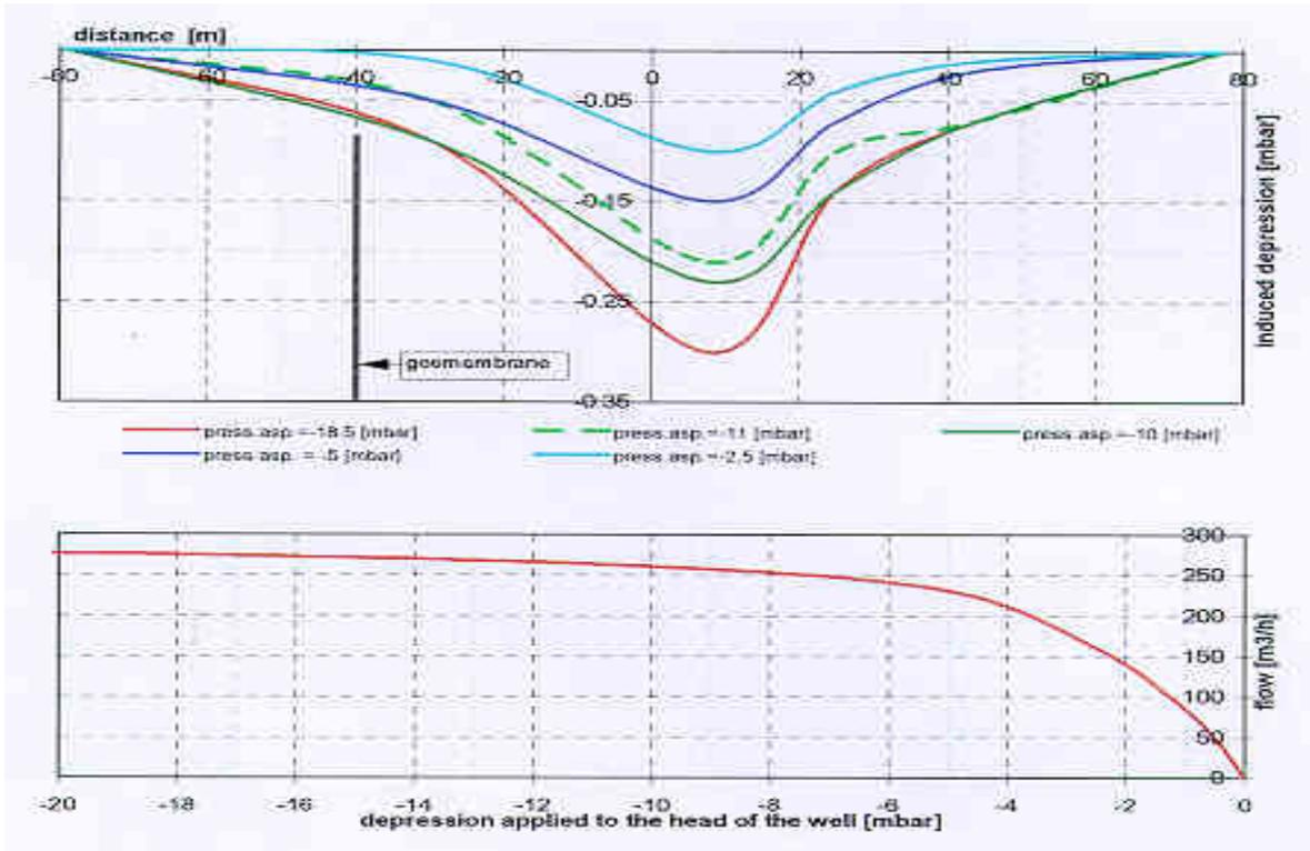
Fig. 10 - Determination of the radius of influence of a well in a natural, permeable soil, and characteristic curve at the well head.
