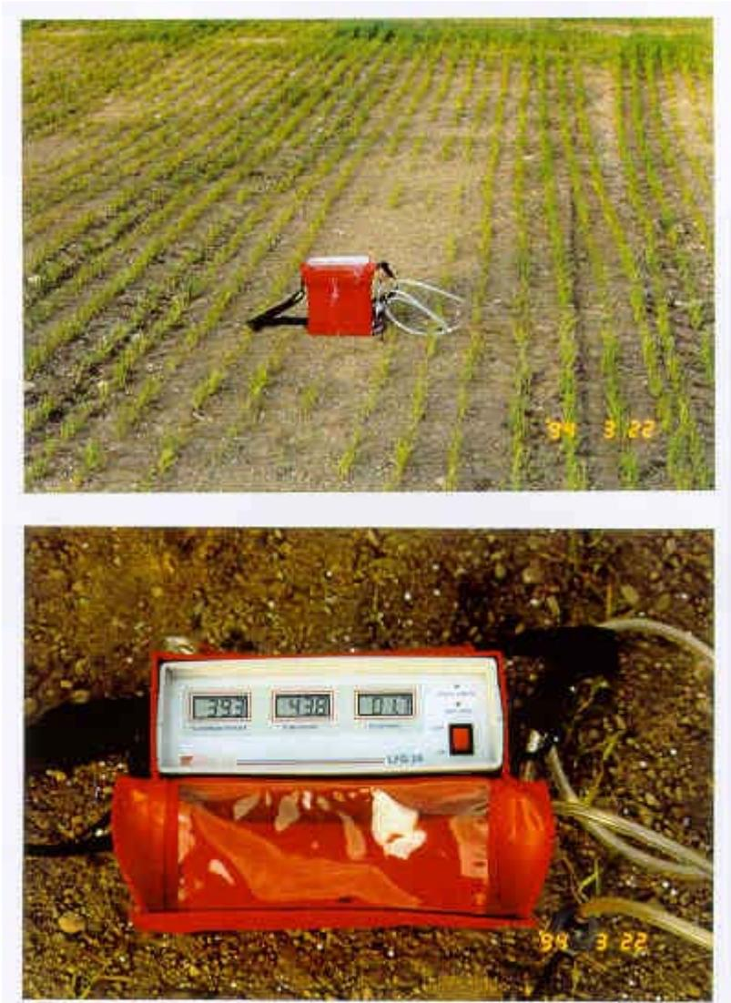
*Fig. 8 - Taking a closer view at the lighter patch visible in the previous photo, evident signs of stress are seen in the corn field west of the landfill. The portable gas detector shows concentrations of almost 40% CO<sub>2</sub> and 44% CH<sub>4</sub>, 10 cm below ground level, explaining why vegetation cannot grow in this area*
