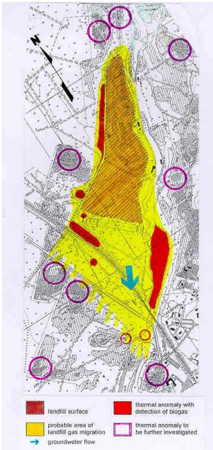
*Fig. 5 - Results of an aerial thermography carried out in 1993 over landfill no. 2 and of biogas detection at ground level, outside the landfill body.*
