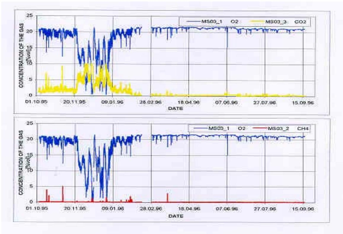
*Fig. 11 - Example of output of an automatic monitoring system. The concentrations refer to a well in a barrier, situated 30 m away from the landfill boundary. The anomalous concentrations measured in December 1995 correspond to an interruption of the internal biogas extraction system of the landfill. The barrier was not started then, to enable the designers to follow the biogas migration path through the monitoring system.*
