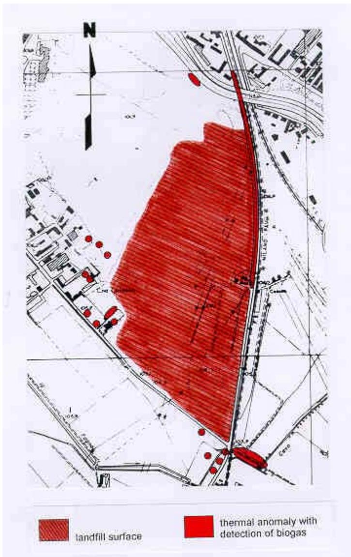
*Fig. 3 - Results of an aerial thermography taken in 1984 over landfill no. 1 and of biogas detection at ground level, outside the landfill body.*
