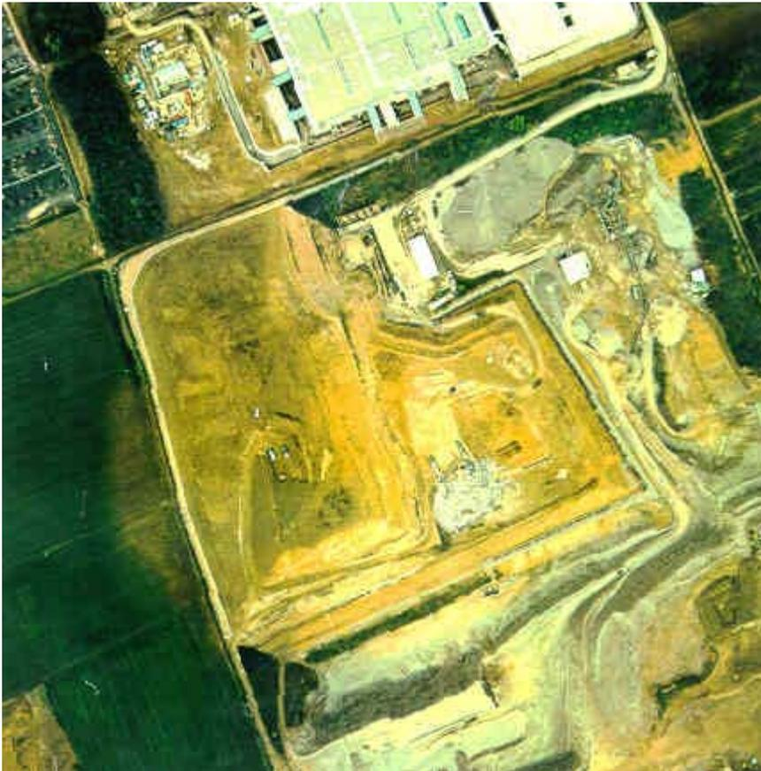
*Fig. 7 - Aerial colour photography carried out in 1994 over landfill no. 3. The lighter patch in the vegetation west of the landfill marks the start of biogas migration outside its boundaries.*
